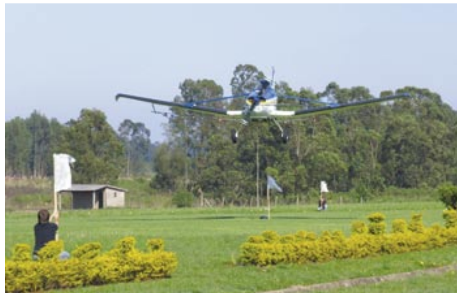
Julio Kampf holds a flag to direct Wagner Patta in his Terra Agricultural Aviation C-188 Ag Truck over the test area to check droplet size.
